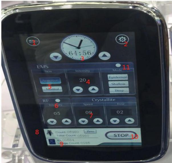
1.tube cleaning 2 language 3 time setting 4 EMS energy 5 skin type 6RF open and energy adjust7 speed 8 account 9 ID card 10 open/close 11 EMS switch
