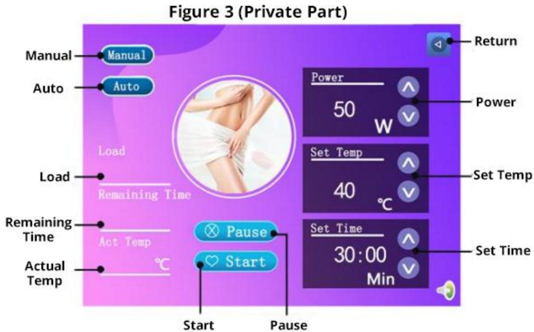
Reminder: If the load displays 00, it means there is no power. There is energy output only when the load displays numbers. If the handle is touching the skin, and the load shows 00 with no energy output, please check whether the cathode pad is installed and connected or whether the cathode pad is touching the customer's back.
