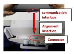
3、Insert the power connector into the connection port
