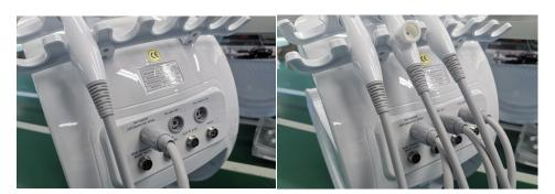
Installation of 2) high-frequency spatula, ultrasonic waveguide head, gold radio head, camera First find the corresponding hand gear connection line and the corresponding plug, the plug groove position is aligned to the left clasp position of the connecting hole, push hard inward, and then tighten the nut counterclockwise after fastening.
