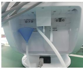
Step 3: Add the purified water (which must be pure water) to the water outlet. After the water is filled, it flows out from the overflow port. Add water to complete
