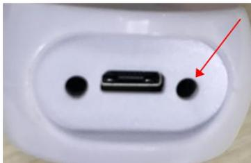
Power Outlet (when operating, insert two connecting cord separately into these two outlets)
