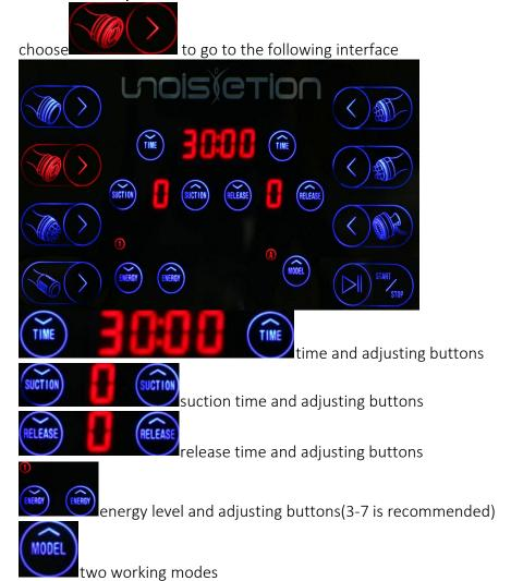
Mode A: the red light goes on and the energy of the handpiece directly reaches preset level after the start button is pressed.
