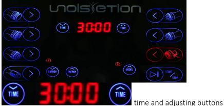
energy level and adjusting buttons(3-7 is recommended)
