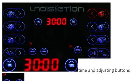
energy level and adjusting buttons(3-7 is recommended)
