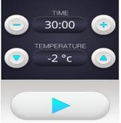
control interface on the cooling applicator
