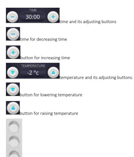
three knobs for adjusting suction levels. Set it at relatively low level at the beginning. When the handpiece is fixed on skin, turn the knob to raise energy level. Do not abruptly raise it to the highest level.
