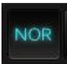
NOR is fixed mode, RF handle directly reaches preset energy level after the start button is pressed.
