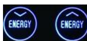
Release Time Setting (the left is for time decreasing and the right is for time increasing)
