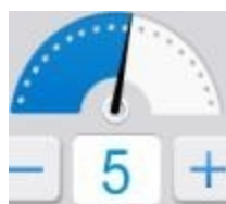
Vacuum Suction Time Adjustment (Suction time > Release time)
