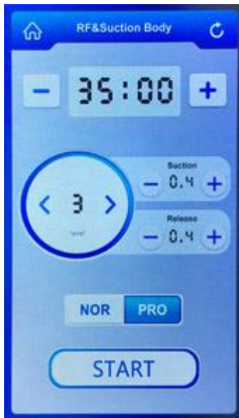
Vacuum Release Time Adjustment (Adjust release time subjecting to one's comfort level; release time is the interval between suction and release; 0 means direction suction)
