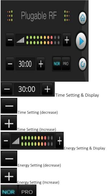
(NOR is default mode. The temperature for RF will reach the setting value directly. PRO is smart mode. The temperature for RF will reach the setting value slowly.)
