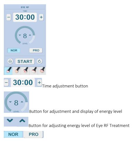
The working mode of eye RF Treatment (NOR is smart mode, LED begins to turn red after touching the skin, and the heat of RF is released slowly to reach the energy setting. PRO is the fixed mode. After pressing the start button, the red LED is always on, and the RF temperature is directly set to the pre-set level.)
