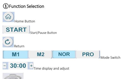
The knob is used for adjusting the suction level of the RF Vacuum. (Twist to the left to decrease the suction level and twist to the right to increase the suction level.)
