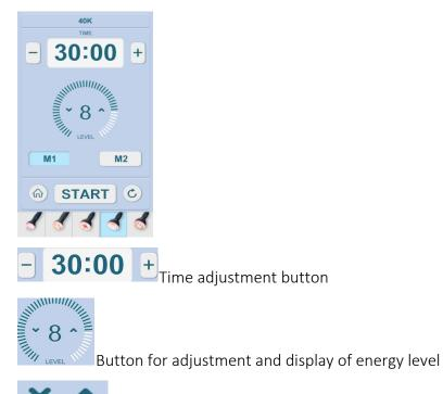
Button for adjusting energy level of 40K Treatment
