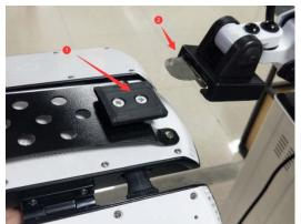
Insert the back of the lamp board (1) into
