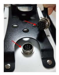
Connect the wire with the jack on the back of the  $\ensuremath{\mathsf{PDT}}$
