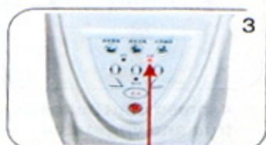
3. The power turns red (indicating normal standby)
