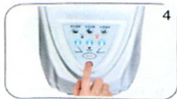
4. (3 seconds after power on) by pressing the power switch, all function lights lit
