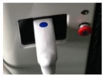
Note:Pls make sure each holes connect well,after connected can hear a sound "DA",
