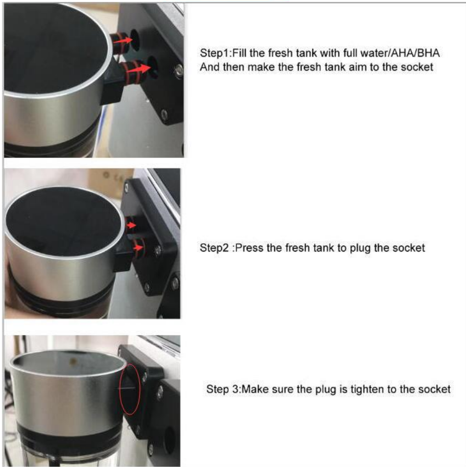
Fig 7.0 Fresh&waste tank installation
