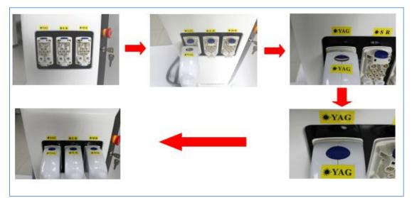
Connect the cavitation and RF handpieces to the connecting port on the left board of the machine tightly.
