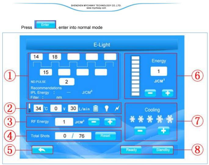
① Parameter status(indicates the first pulse, delay, pulse number and time)
