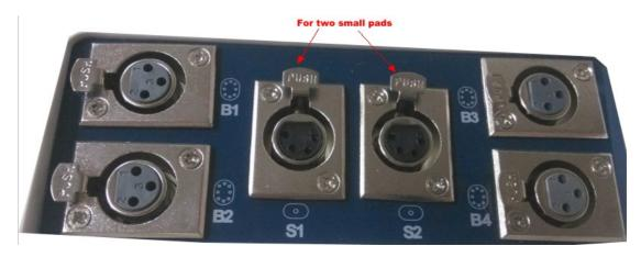
S1,S2 is for two small pads,4pin jet.
